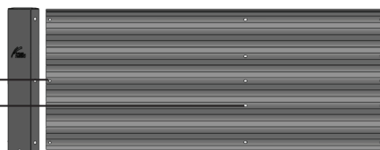
Fig. 2 Use the edge with 3 holes to assemble the corners
